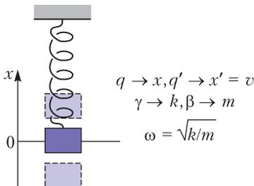
$$\begin{aligned} q &\rightarrow x, q' \rightarrow x' = v \\ \gamma &\rightarrow k, \beta \rightarrow m \\ \omega &= \sqrt{k/m} \end{aligned}$$
